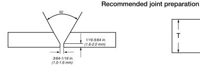
Wall thickness <3/4 in. (<20mm)
